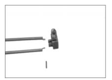
Separate Springs(022) and Block(028) by taking away Rod(025).
