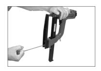
When *Anvil(029)* is properly aligned, tighten pivot *Screw(521)* first, then tighten retaining *Screw(514)*.
