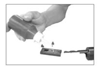
Reassemble New Driver Guide (016) and *Screws(520)*. NOTE:Use Locktite soluent #75559, apply Locktite grade 277.
