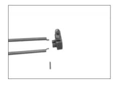
Separate *Springs(022)* and *Block(028)* by taking away *Rod(025)*.
