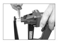
Insert single staple into *Driver Guide(016)*, leaving points protruding.
