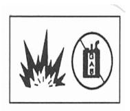
NEVER USE GASOLINE OR OTHER FLAMMABLE LIQUIDS TO CLEAN THE TOOL. VAPORS IN THE TOOL WILL IGNITE BY A SPARK AND CAUSE THE TOOL TO EXPLODE AND RESULT IN DEATH OR SERIOUS PERSONAL INJURY.
