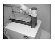
GRASP HANDLE WITH ONE HAND POSITION ON BOX IN LINE WITH THE DESIREDSTAPLE LOCATION.
