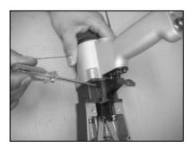
LOOSEN SCREWS (025) WITH FLAT SCREW DRIVER . AND REMOVE TRIGGER ASSEMBLY (024).
