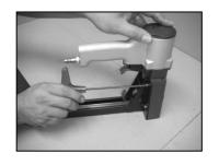
LOOSEN SCREWS (530) WITH 4  ${\tt mm}$  HEXAGON WRENCH KEY .
