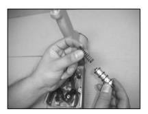
REMOVE VALVE (032) AND TUBE (031) WITH A LONG NOSE PLIERS.
