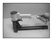
DISCONNECT THE AIR SUPPLY FROM THE TOOL.
