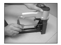
LOOSEN SCREWS (530) WITH 4  ${\rm mm}$  HEXAGON WRENCH KEY .
