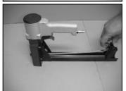
PULL PUSHER (034) BACK UNTIL IT STOPS ON STOPPER (038) THEN ROTATE PUSHER (034) TO POSITION .
